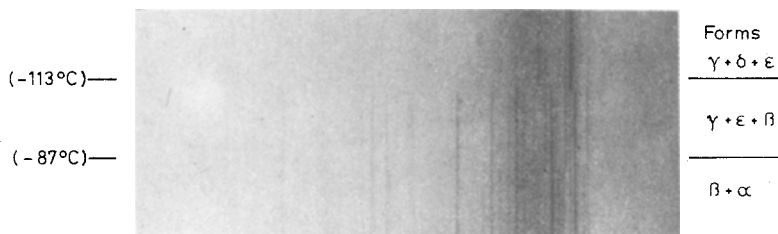
Fig. 5 Guinier-Simon diffraction experiment (heating pattern of cyclohexane as a microsample in an emulsion)
